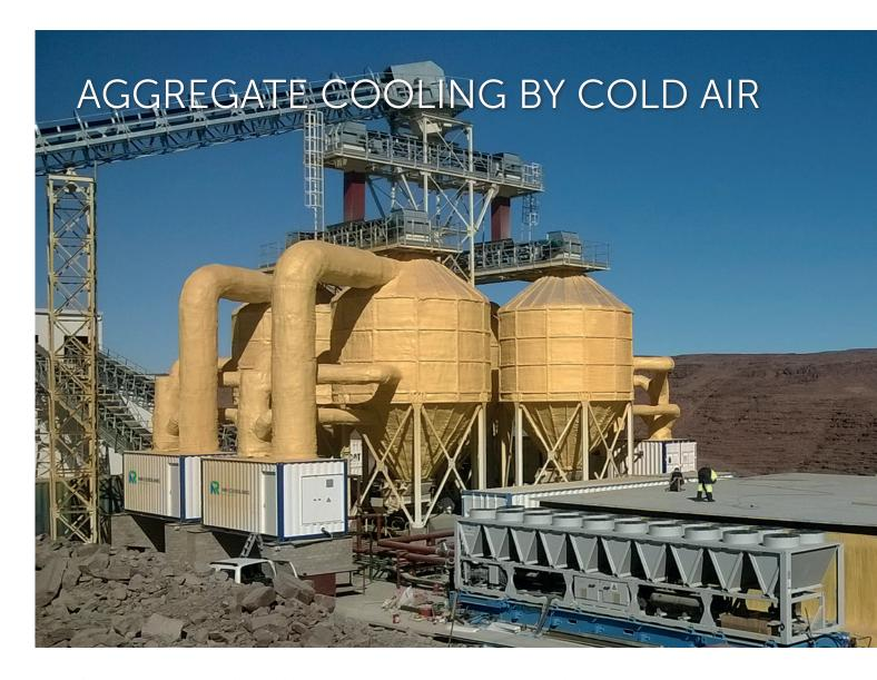
Concrete consists of 40% to 60% aggregate with sizes of 5 mm up to 150 mm. When high concrete production rates and extreme temperature reduction are required, cooling aggregate by air has proven to be very effective. When using this technology, the limitation of added water is not a limiting factor in reaching the desired concrete temperature. This means that lower concrete temperatures can be reached compared to other common systems.
