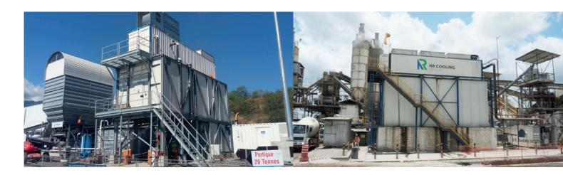
The most frequently applied cooling method for lower fresh concrete temperatures is replacing the mixing water by flake ice.
